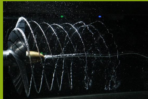
Tip and hub vortex cavitation on a ship's propeller.
