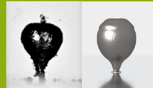
Single bubble collapse near the wall: Experiment (left) and simulation (right).
